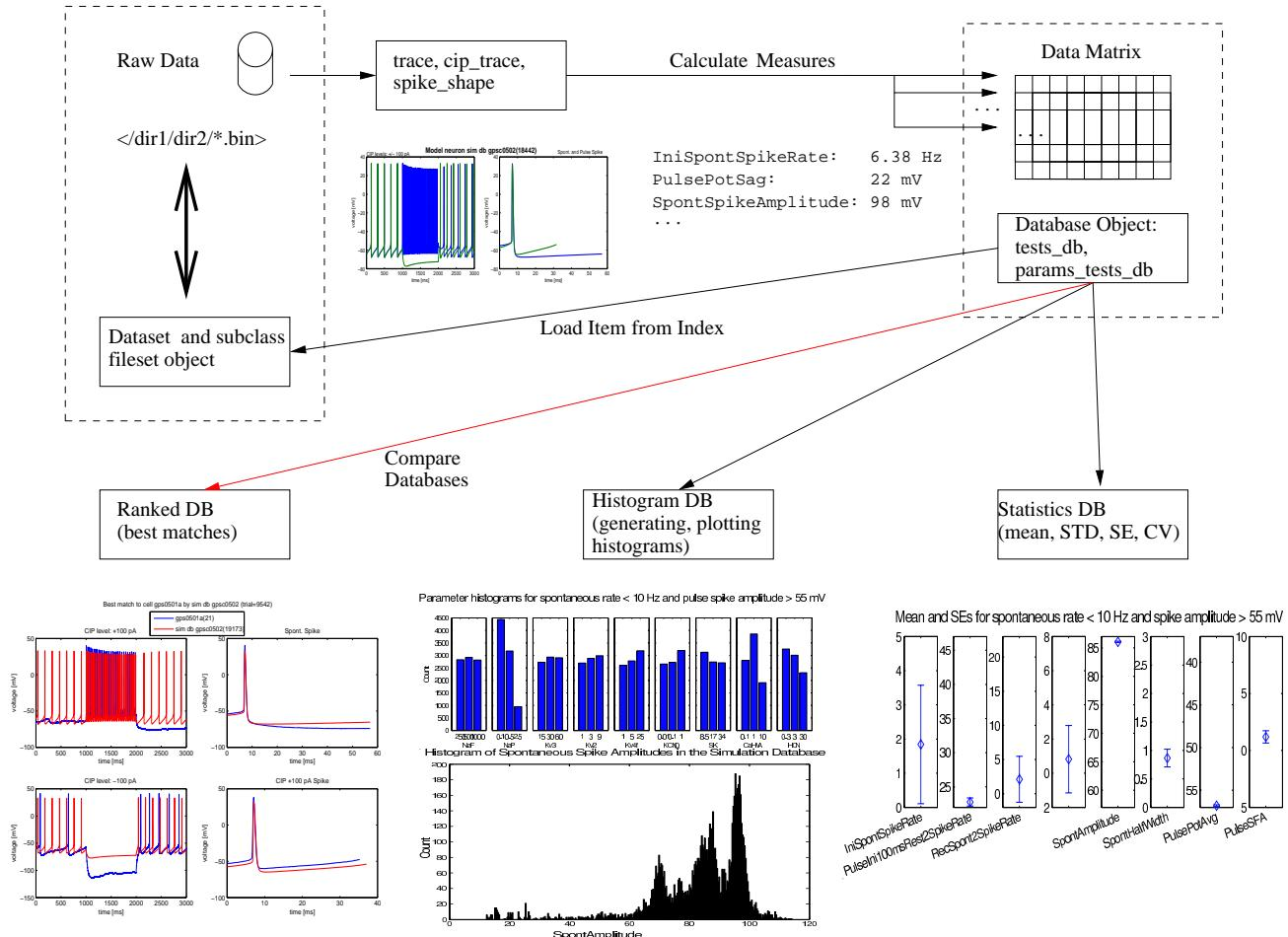
Figure 1: Schematic overview of the database software.
